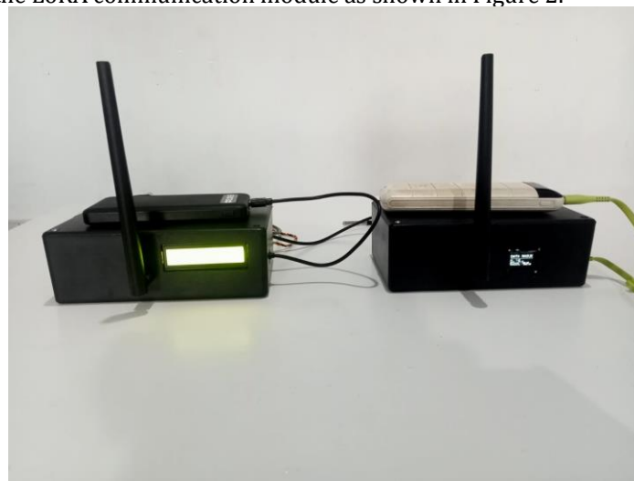
Figure 2. Sensor Node and Gateway Devices
