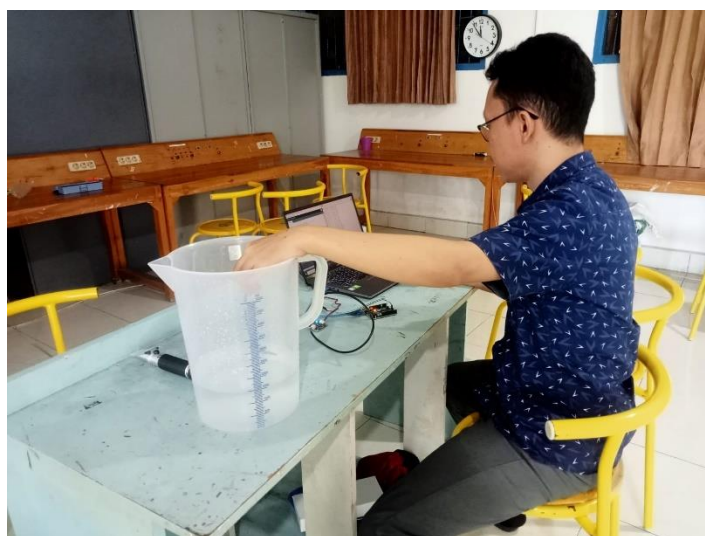
Figure 5. Water Salinity Measurement with TDS Sensor
